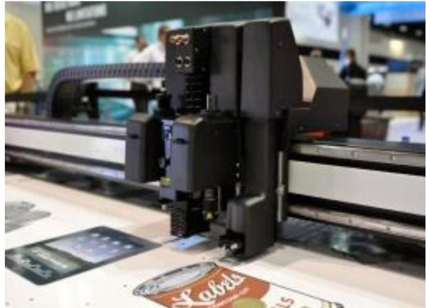
In these modules, several tools can be mounted, e.g. a static knife, a pressure controlled knife or a creaser (to make folds in cardboard). With these tools it's possible to cut a whole range of materials up to several millimeters thick: roll-material, plastics, cardboard, foam board,... Of course Summa plans to expand its toolset to boost the capabilities of the flatbed machine and approach other cutting applications.
