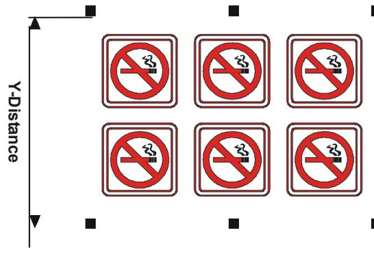
**CAUTION:** The exact distance between any two markers along the X-Axis or Y-Axis must be established. Measure this distance in the design software, not on the media!
