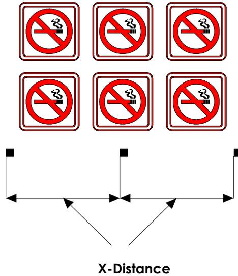
**NOTE:** OPOS will operate faster as the X-Distance increases. Conversely, OPOS will operate more accurately as the X-Distance decreases, however this impact on accuracy is minimal.
