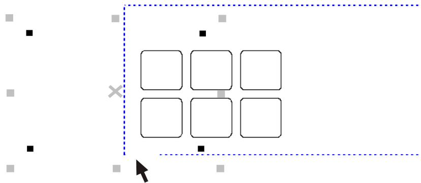
**HINT:** Some software will shift the selected contours to the Origin when cutting. This can be avoided by adding a small rectangular spacer that has its bottom left corner in the Origin. Select this rectangle along with the contours.
